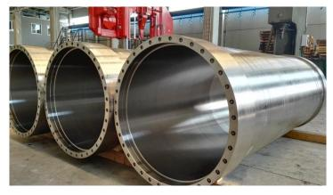
1350mm, lengths up to 1250mm. Vertical centricast items are normally shaped, but we can produce also simple cylindrical rings.
